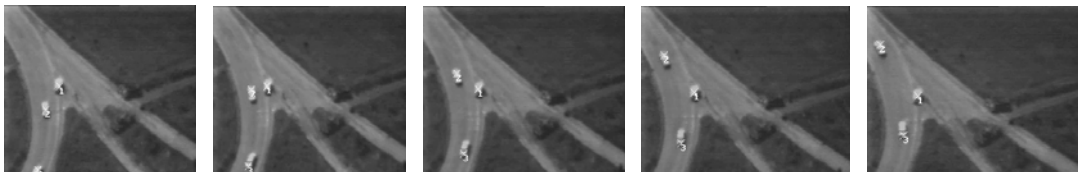
Figure 5: tracking multiple targets simultaneously from an UAV platform.
